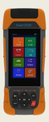
GW1000 SmartOTDR series adopts a 3.5 inch color capacitive touch screen, which enables rapid and hand-free operation . It combines eight essential fiber tests in one handheld with OTDR, event map, stable light source, optical power meter, red light source, network line sequence test, line finding and lighting. Simple parameter setting and intelligent measurement ensure the operation more simple and efficient .
