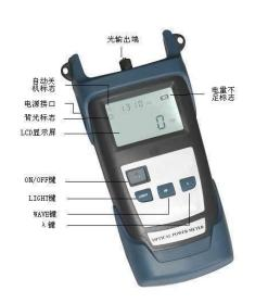
the icon "AUTOOFF" appears in the screen, the device will automatically turn off if there are no operations within 10 minutes. If the icon "AUTOOFF" doesn't appear in the screen, it indicates that the
